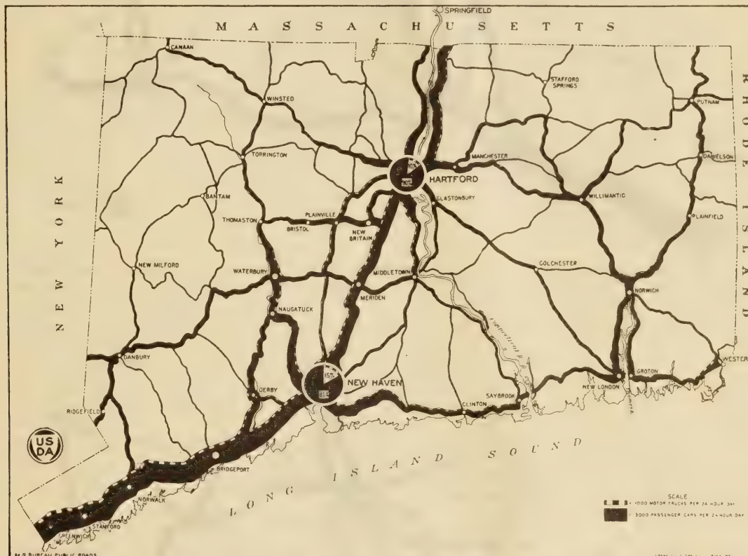
Fig. 2.—Average daily movement of motor trucks and passenger cars on the Connecticut highway system.
